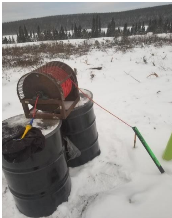
Figure 1: Illustration of the spool and the wireline holding the fluorometer.
