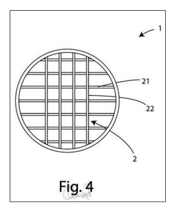
A plurality of tubular canals (Fig. 4) divided into horizontal and vertical lines covering the entire surface of the helmet.
