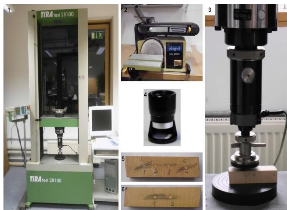
Figure 7: Hardness test methodology: 1.TIRA test 28100, 2.Sandermachine, 3.Press of the steel ball into wood sample, 4. Micro loupe, 5. and 6. Indentation point in cross and radial sections, respectively.
