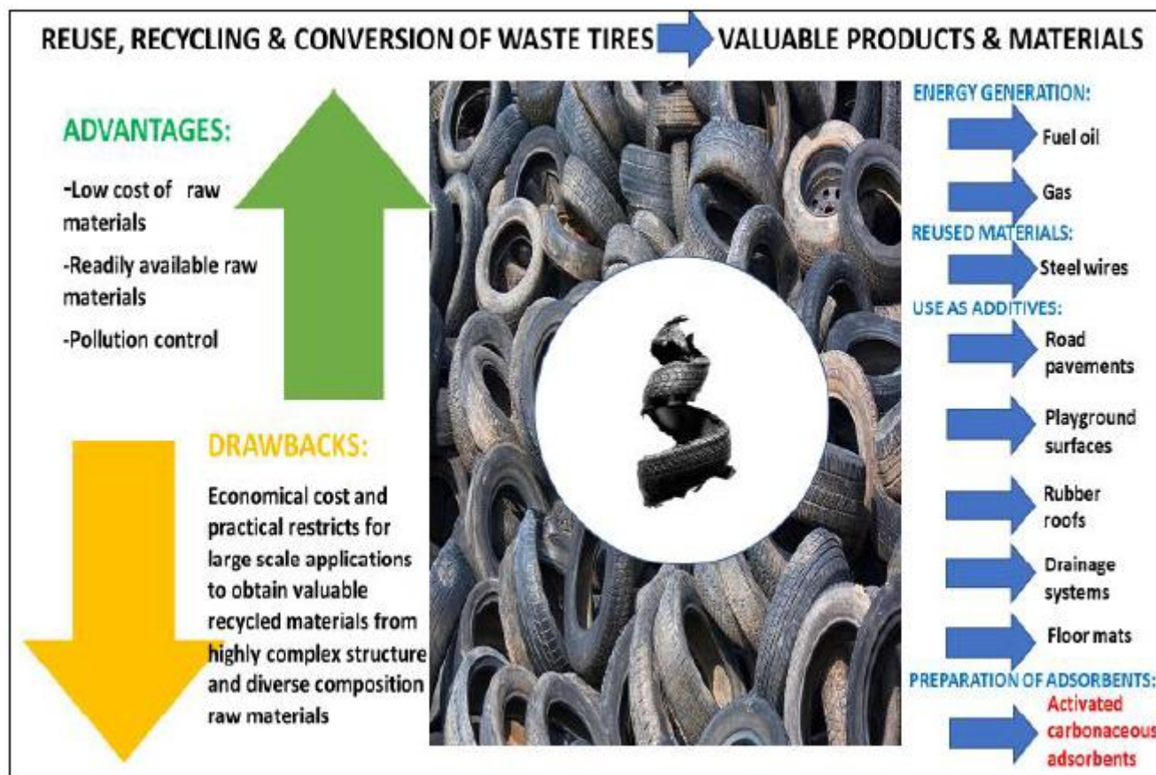
Figure 1. Some examples of reuses, and recycling or conversion strategies of waste vehicular tires.
